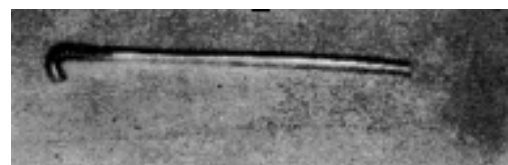
Dent rod for bottom bow of sax bodies.
