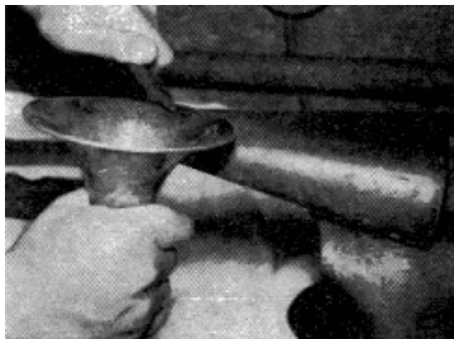
Use of bell iron and burnisher to remove dents up to the rim.
